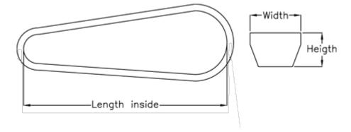
$\begin{array}{ll} \text{Datum Llength} = 970 \\ \text{Height} & = 6 \\ \text{Length inside} & = 950 \\ \text{Width} & = 10 \\ \end{array}$
